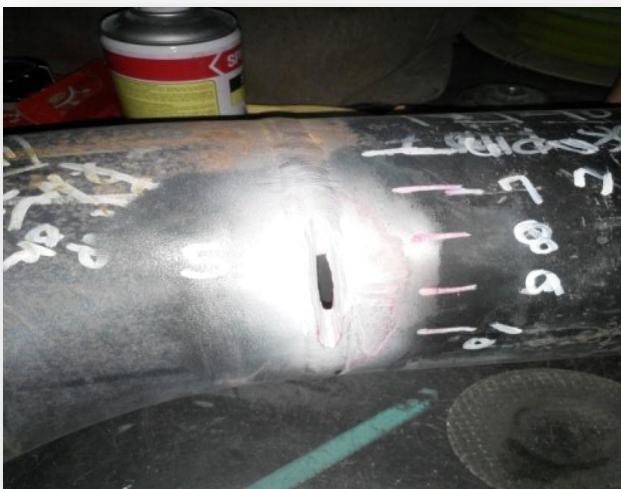
Fig 2. Pipeline Showing Crack with Measurement (Picture Courtesy-SADARA, KSA) A diagram showing the implementation of an edge detection algorithm.
