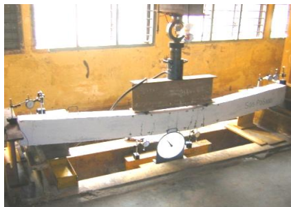
Fig. 6 Failure Mode of SFRC Beam
