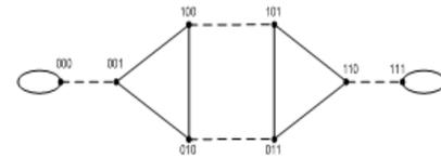
Figure 1 The 8 - node Shuffle Exchange Network
